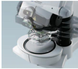
The motorized lens blocking process takes only two seconds, greatly increasing productivity. Since excessive blocking pressure can cause lens coating deterioration when the block is removed, the Ice 900 applies the appropriate blocking pressure, and protects lens from the damaging. In addition, the block adapter is ideally positioned for easy and comfortable block loading.
