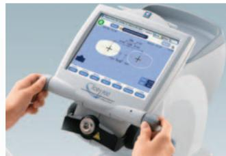
In addition to the intuitive operation of touch screen, data can also be entered by the use of the twin "quick jog" dials. The left jog dial moves the cursor for layout and grinding condition selection, while the right jog dial is used to enter numerical values/changes.
