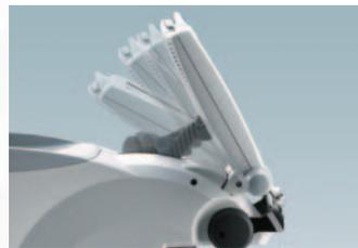
A unique tiltable display allows the LCD operation screen to be viewed at four different angles, making it ergonomically friendly whether in a sitting or standing position.
