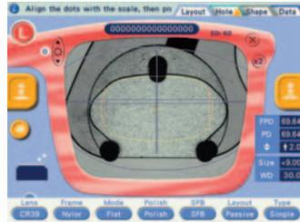
"Smart screen" design provides the operator with an information bar and on-screen tutorial for ease of use. In addition, layout and grinding conditions are easily entered on the color-coded 8.4-inch SVGA touch screen display.
