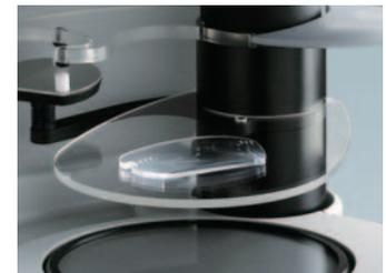
The ISI function detects any demo lens or pattern, including those for rimless drill mounts, and identifies hole position. Moreover, the ISI function automatically compensates horizontal axis. The operation is supported by a "Wizard Tutorial" directly viewed on the screen of the unit, featuring user-friendly instruction.
