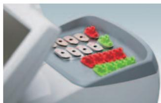
An accessory tray is provided to store small items. The Integrated Shape Imager table, spare fuses, and small-diameter lens holder are all stored under the tray.
