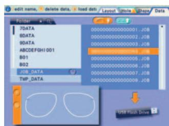
The data management feature allows storing, searching, and recalling of traced data. A maximum of 30,000 patterns can be saved. Data can also be saved to a USB flash drive (optional).
